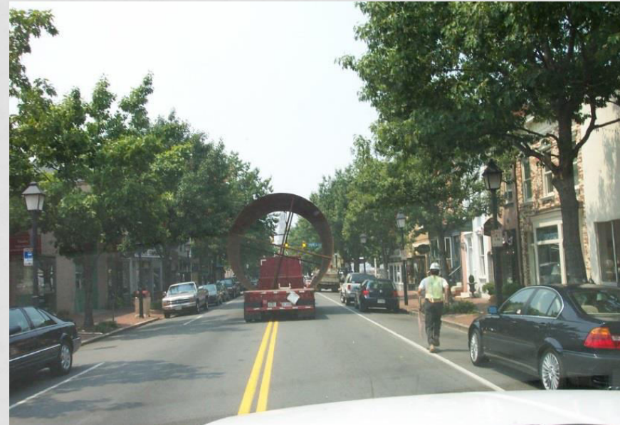
Transportation of the pre-fabricated metal shaft liners.
